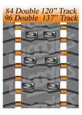
**137"/348cm track** –Use the 286T-TEMP 126/144 Double/Single stud pattern for a 4-2, 4-2, 4-2 pattern. This option will give you a total of 144 studs in the center belt.
