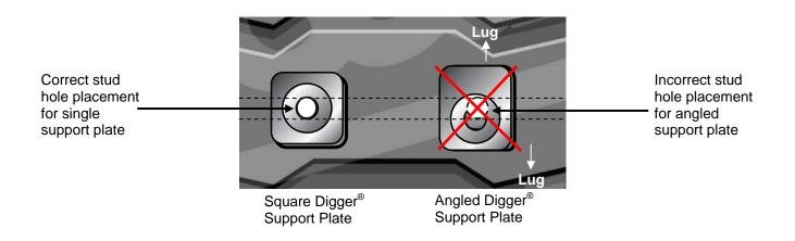
**Do Not** enlarge the hole in the track in an attempt to install Angled Digger<sup>®</sup> Support Plates on Camoplast Preholed tracks.
