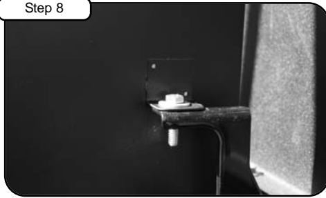
Install screws with washer though tab. Using washer, wavy washer, and M6 nut place on other side of screw.
