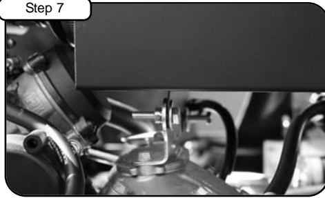
To install housing into Teryx guide into coupler and position to bracket. Use screws, washer, and wavy washer to bracket. Tighten using 10mm socket or wrench.
