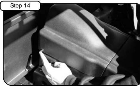
Install air box cover using push clips. Your installation is now complete. Please check all bolts and clamps periodically. Re-tighten if necessary. Thank you for choosing aFe!
