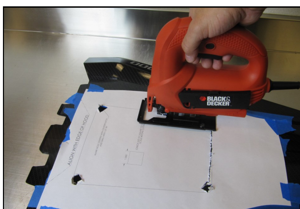
23. Using a jigsaw or equivalent, cut along the template line and connect the 1/2" holes. Remove the hood center and the template.
