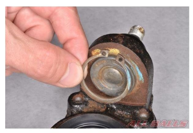
Remove the snap ring with snap ring pliers.
