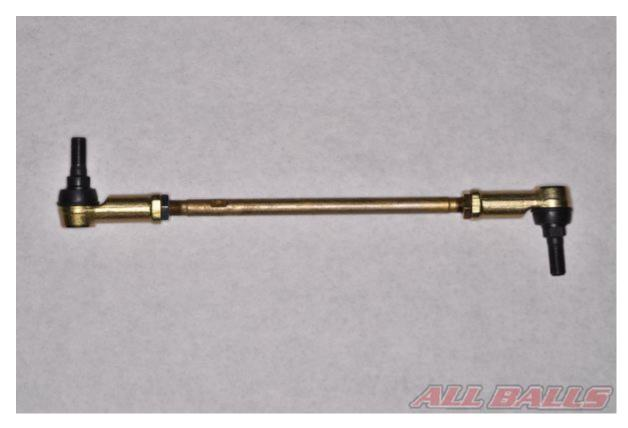
Set the position and distance between the tie-rod ends according to the OEM requirements.
