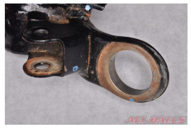
Clean away all of the old grime and rust from the ball joint bores. Remove any burrs that may inhibit the installation of the new ball joints.
