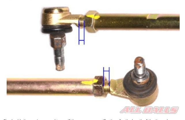
Check with the service manual to see if there are any specifications for the length of the tire rods or the amount of threads that should be showing. If the tie-rods are not adjusted according to the OEM specifications the proper toe-in may be achieved, but the vehicle will not steer correctly and it could be at risk of breaking a tie-rod.
