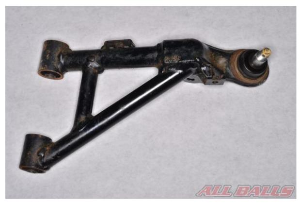
Remove the A-arm. See the vehicle's service manual for specific information.
