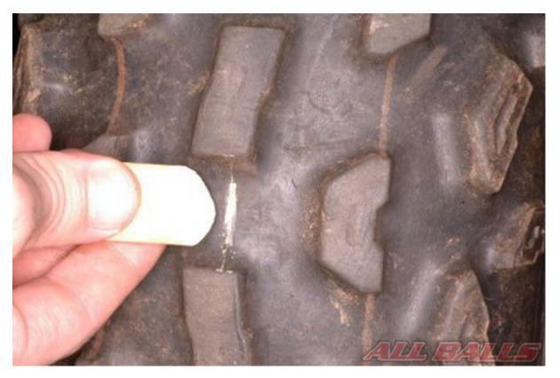
Make a chalk mark on the front, center of each front tire at the height of the front axle. If available set up a toe gauge so that the pointers line up with the chalk marks.
