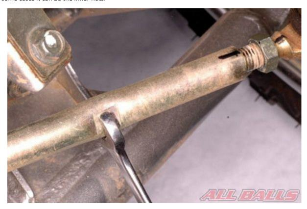
Turn the tie rods with a wrench at the flats to change the toe-in. Evenly adjust the left and right tie-rods for proper alignment.
