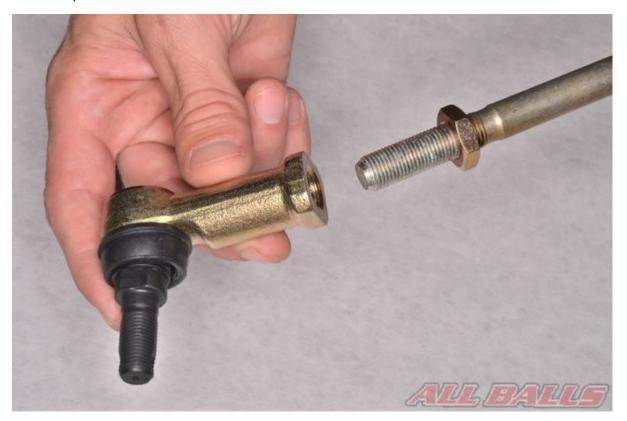
Install the tie-rod end onto the rod.
