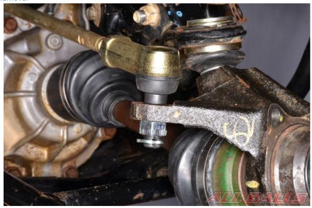
Remove the tie-rod nut cotter pins.
