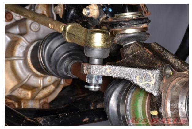
Install the tie-rod to the steering shaft and knuckle. Make sure the ends are positioned correctly so the ball joints are not at severe angles. Install new cotter pins with the ball joint nuts.
