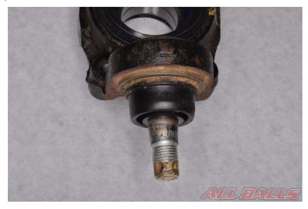
Spray the tapered portion of the ball joint with a penetrating lube to aid in freeing it.
