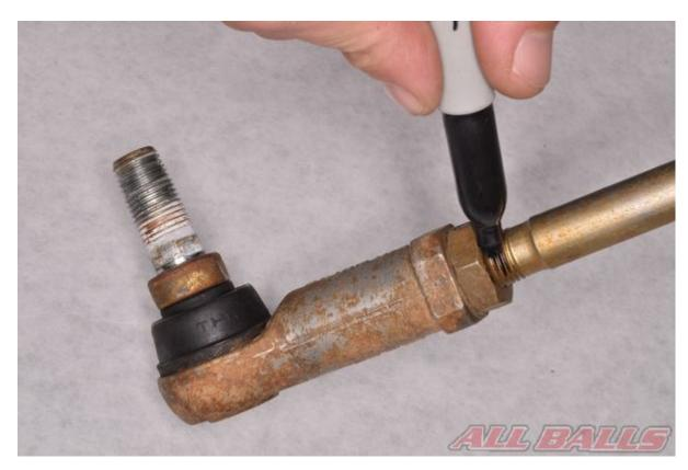
Mark the tie-rod for a starting point for reassembly.
