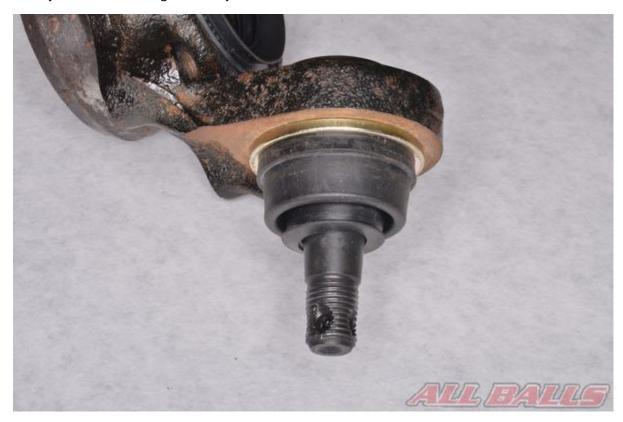
Make sure the ball joint is fully seated and the boot has not been damaged.
