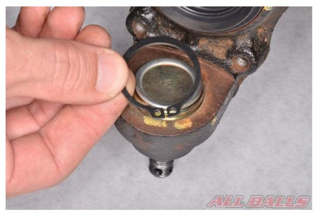
The snap ring groove should be visible.
