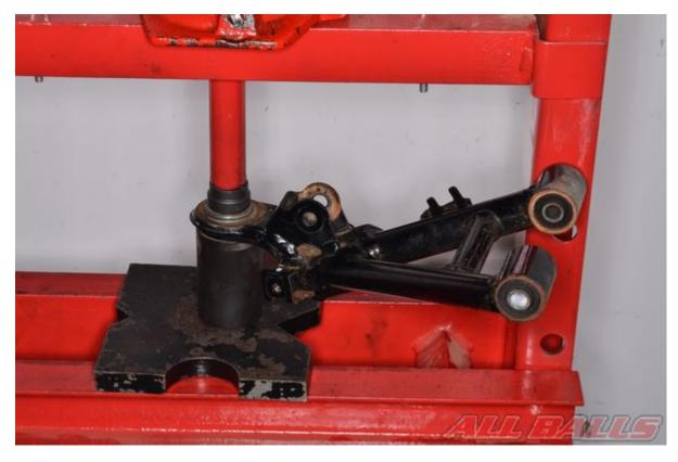
Use a press and appropriate tools to press the ball joint out of the A-arm. Make sure the ball joint has room to exit the A-arm.
