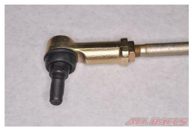
Tighten the lock nut against the tie-rod end to set the position.
