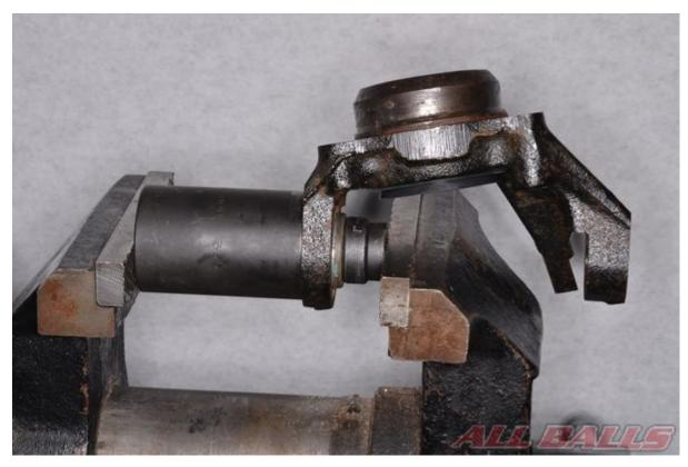
Use a vise and appropriate tools to press the ball joint out of the knuckle. Make sure the ball joint has room to exit the knuckle.
