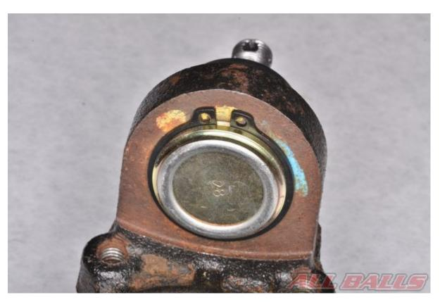
Install the new snap ring into the snap ring groove.
