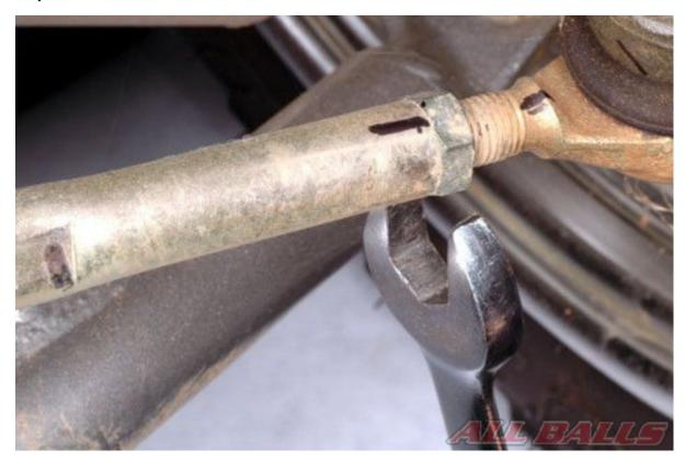
The outer or inner tie-rod lock nuts must have reverse threads. Usually it is the outer nuts, but in some cases it can be the inner nuts.
