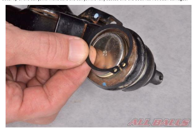
The snap ring groove should be visible.
