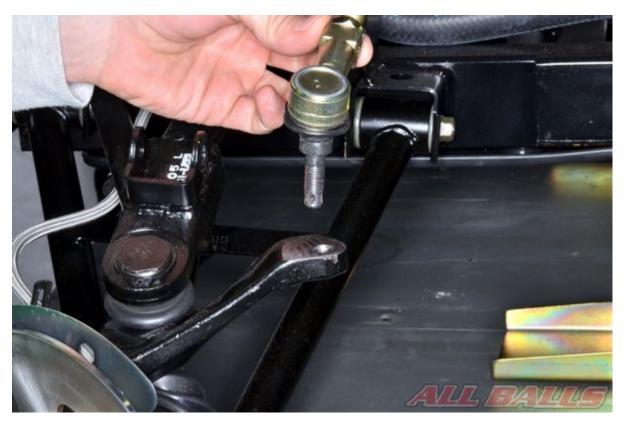
Free the tie-rod from the knuckle and steering shaft. See the vehicle's service manual for specific information.
