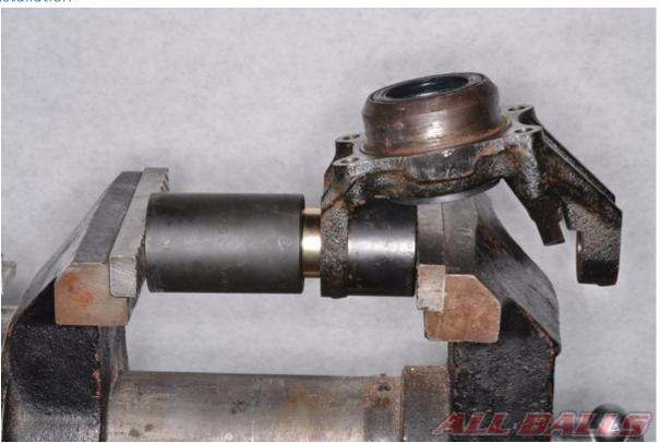
Install the new ball joint into place. Use a suitable tool that will only contact the metal outer lip of the ball joint. Do not damage the ball joint boot.
