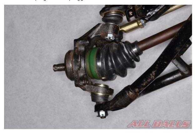
Install the knuckle to the suspension arms, tighten the nuts to specification and install the new cotter pins.
