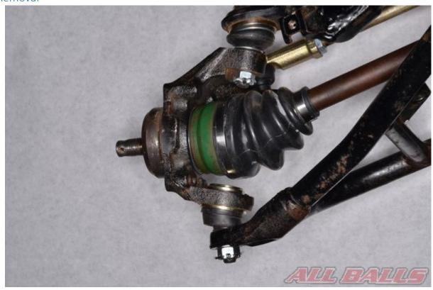
Remove the wheel hub and brake assemblies from the knuckle. See the vehicle's service manual for specific information.
