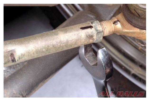
When the adjustment is correct hold the tie-rod flats and tighten the lock nuts to specification against each side of the tie-rod. Take a slow test ride to make sure the steering functions correctly.
