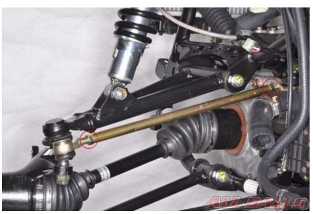
To adjust the toe-in loosen the lock nuts on the tie-rods.
