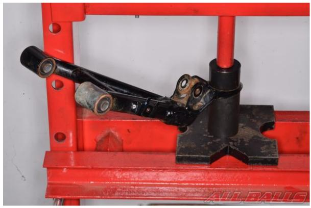
Install the new ball joint into place with a press. Use a suitable tool that will only contact the metal outer lip of the ball joint. Make sure the ball joint is fully seated and the boot has not been damaged.
