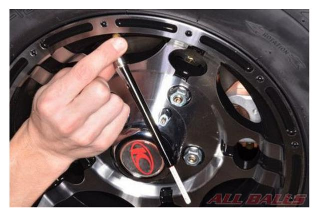
The first step in checking the toe-in is to check the tire pressure. Make sure the tire pressure set correctly in all four tires. The air pressure in the front tires should be as close to the same as possible.
