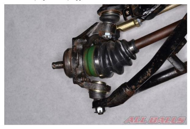
Install the suspension arms, tighten the nuts to specification and install the new cotter pins.
