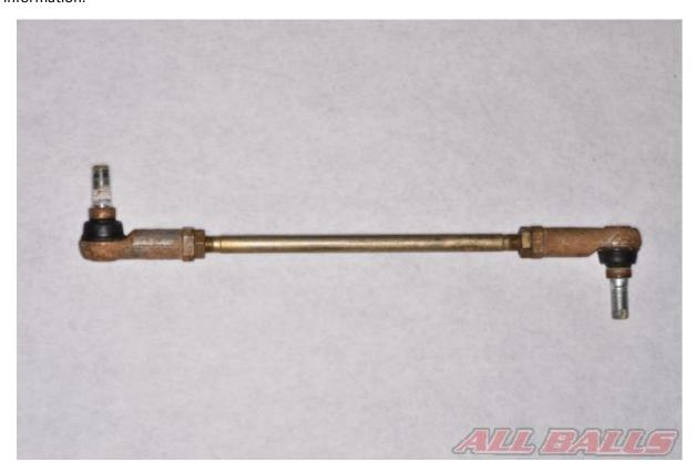
Inspect the tie-rod for wear and damaged. Note the position of the ends. Some vehicles have specific instructions for tie-rod length and end positioning. Check the service manual for the specific information for the vehicle.
