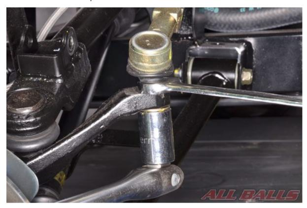
Remove the tie-rod nuts. It may be necessary to hold the tie-rod with a wrench when loosening the nut.
