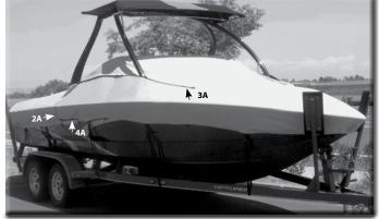
in the envelope-type pouches at the hem on each side of the cover. Refer to Rope Ratchet Instructions to tighten the draw rope. When draw rope is tight, close each pouch over the ratchet.
