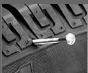
Puncture – Normally, the only evident of a puncture will be a cut that extends from the tread of the tire through the inner liner.
