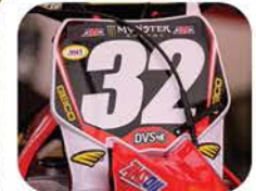
Stadium Number Plate Lighter Than Stock Includes Cable Guide
