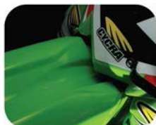
Powerflow intake channel routes air to radiator
