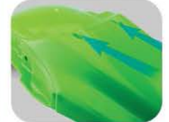
Powerflow Rear Fender Provides Clean Airflow to Airbox
