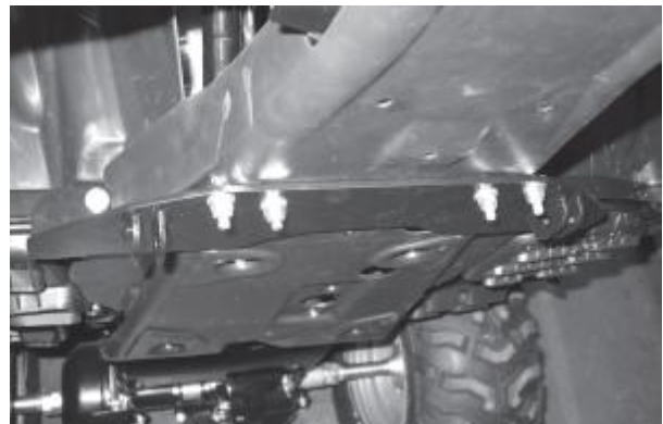
Figure 9 - Plow Mount Installed
