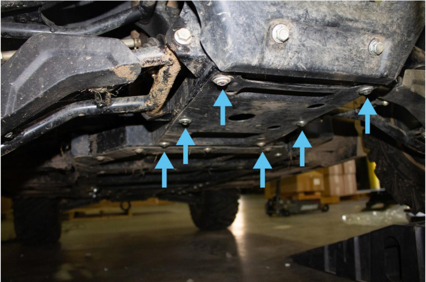
2. Place each threaded bracket behind the two holes in front and behind the differential.
