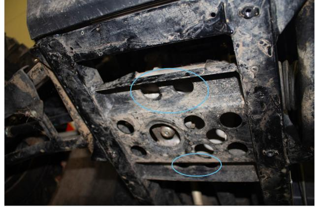
3. Hold mount to frame and insert provided bolts to threaded brackets using a washer and lock washer on each bolt.
