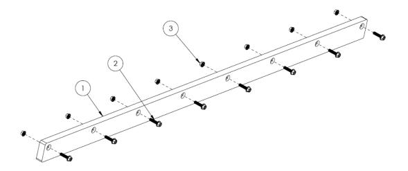
Install the Urethane Wear Bar (#1) to the bottom of the Plow Blade using the  $3/8 \times 1.5$ " Serrated Flange Bolts (#2) and 3/8" Serrated Flange Nuts (#3) included in the Polyurethane Wear Bar kit.
