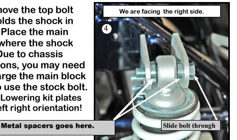
3) Bolt both plates to the main body. Leave the nuts off for now. Holes determine bolt size you will use. 4) Slide the bolt through the hole of the plate and then through a spacer. The bolt will now pass through the hole of the shock. Put another spacer in and now
