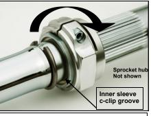
3) Slide the c-clip into the groove on the axle (hub not shown).
