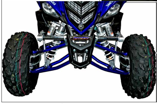
3> Once everything seems to be aligned, tighten all the clamps and bolts. This is how the finished installation should look. Bounce the front end up and down a few times to make sure there is no binding or rubbing. If you need to loosen some of the clamps and realign, do so.
