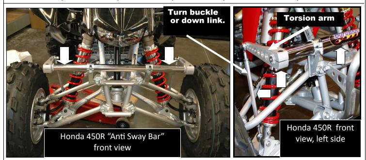
The Anti-Sway Bar is a universal kit that will fit almost all ATV's. The kit is designed for easy installation, but can be modified to fit where ATV upgrades have been added, making normal installation more difficult. The kit can be adjusted to preload one side which will add greater stability when racing on tracks with all right or left hand turns. (see page 2) Most riders who flat track race have these kits. Please consult the application as some AT-V's have their own dedicated kits.
