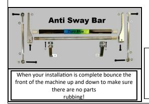
General rules to mounting The Anti-Sway Bar The tube housing can be mounted on the front of the frame or the behind the a-arms. The torsion arms should be parallel with the ground, and the turnbuckles should as perpendicular to the ground as possible.
