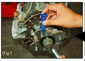
Squeeze a drop of Lock-tite at the base of the wheel stud threads. Don't coat the entire thread stack, just the last few-threads.
