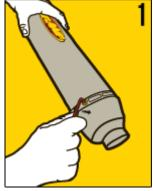
Before getting started with the repack, be sure to remove any spark arrestor or insert from the muffler outlet. To begin repacking, first remove the Allen screws from the front of the muffler (closest to the midpipe). Do not remove the rear end-cap from the muffler can.
