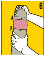
Slide the inner core assembly into the canister, making sure it is fully seated into the rear end-cap. Wipe off any excess silicone and reinstall the Allen screws. Tighten each screw an additional 1/4 turn once the screw has made contact with the canister. Allow sufficient time for the silicone to cure before starting the engine.
