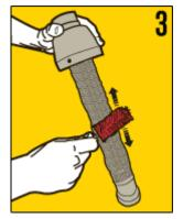
Unwrap the old packing from the core and discard. To ensure there are no clogs in the perforations, clean the core with a wire brush to remove all of the old material.
