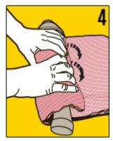
Align the new packing with the longest dimension running the length of the core. Wrap the core and secure the packing with a strip of ½" wide masking tape near each end. The packing should be snug, but not too tight, as this may actually increase the noise level.
