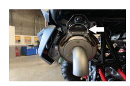
3. Remove the three bolts securing the hanger shield, then remove rubber insulator and then the shield. Next, remove the factory muffler by sliding it off the driver side hanger. Use WD-40 to lube the rubber insulators to aid removal.
