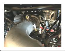
2. Remove the two factory bolts with springs from the headpipe and set aside to re-use later. Do not damage the factory exhaust gasket. You will re-use this gasket. Then loosen the O2 sensor and lay it aside for later re-installation.
