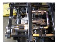
7. Now install the Gibson muffler and slide hanger rods into grommets. Then install the 3 supplied exhaust springs from the muffler to the midpipe.
