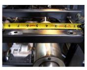
5. Now in the rear frame of your Rhino, you need to drill 2 3/8" holes. The first hole should be 11/4" and the second should be 7 1/8" from the right side of the frame inside of the bed mount bracket
