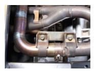
3. Now install Gibson mid-pipe onto stock header using supplied 1¾" band clamp. Then install stock band onto Gibson mid-pipe for extra support.
