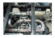
5. After muffler and mid-pipe are in place double check all springs and bolts are in place and tight.
