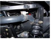
1. Remove the factory muffler by using the 15mm wrench or socket at the band clamp shown in the photo. Spraying a small amount of WD-40 will help with the removal of muffler from the rubber hangers
