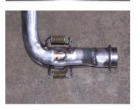
5. Use the factory springs to attach Item C to the header pipes. Item C the collector will have a top and a bottom. When looking at the collector from the side one way will have the single exit facing up wards at about a 10 degree angle or down ward. You want the single exit of the collector facing downward when slipping it onto the header pipes.
