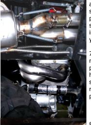
6. With the header still loose, but the header bolts installed attach the supplied Gibson springs. Use the Needle nose pliers and a small flat head screw driver to assist with the install. It is important to use your safety goggles.
