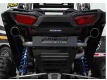
been installed and tighten install your supplied Gibson tips. Slide the tips on to your desired look and tighten down. Check for 1" clearance and go have fun.
