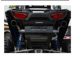
6. Install rear Gibson beauty plate. Use the factory bolts and supplied nylock nuts for the top two holes. Once they have been installed tighten the Gibson brackets at the Razor frame. Adjust plate for a level finish.
