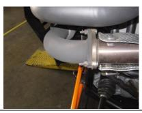
4. Next install the Gibson Muffler assembly. Install the top hanger mounts first then slide the inlet over the factory head pipe re using the factory gasket and nuts. Once in position, install head pipe and top muffler springs.
