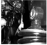
3) On the right side of the ATV, where the top of the shock connects to the frame there is a wire hook that holds a connecting clip. You will need to unhook the clip from the wire hook. With a pair of pliers, mash the clip flat.
