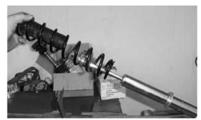
5. Insert the larger rear spring stiffener onto the shock with the lip of the of the spring stopper, on
