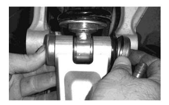
3. Using a shock spring compressor, compress the spring on the shock and remove the spring retaining ring.
