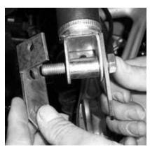
3. Insert the 6x45 hex bolt with the 6mm washer into the front of the brackets sliding in through above the spacer and securing it with the 6mm washer and lock nut on the backside. Note: Once the 6x45 hex bolt is installed fasten it tight, then fasten the 10x50 bolt tight.
