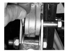
5. Completed view of the shock mount bracket and the spring stiffener.
