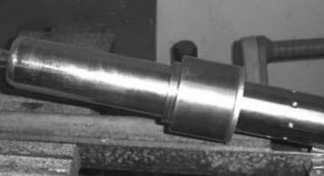
6. Slide the spring back onto the shock and it should rest on the lip of the spring stiffener.
