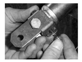
4. Secure the shock with the bracket attached to the shock mount on the A-arms with a 10x50 hex bolt. Place a 10mm flat washer between the bracket and shock mount. Fasten with the 10mm lock nut.
