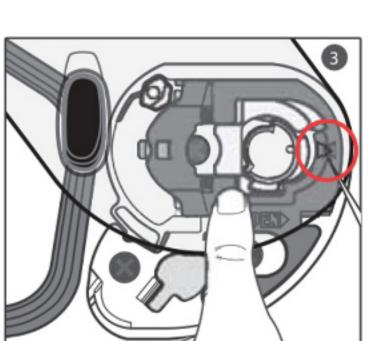
3. With the guides properly aligned, press the lower section of the shield into the plate-gear mechanism. The locking tab should pop into position, locking the shield into place.
