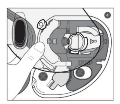
4. The shield will be automatically released out of base ratchet mechanism.
