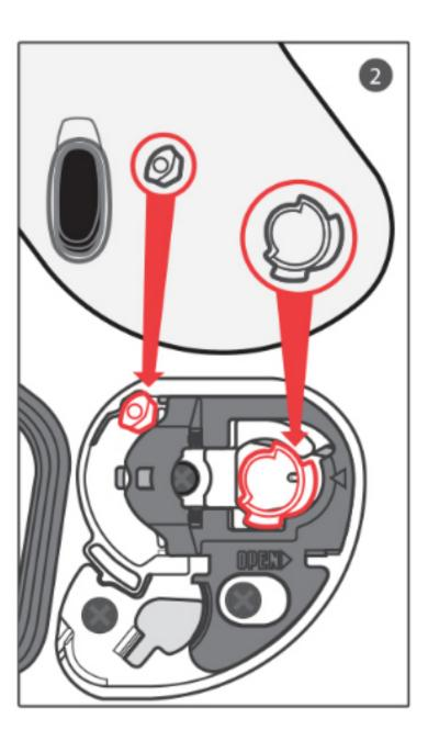
2. Align and insert the top of the shield guide into the plate-gear guide.
