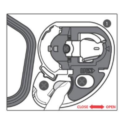
1. Ensure that the handle-locker is in the open position.
