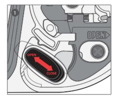
1. Move the shield retention button to the open position.
