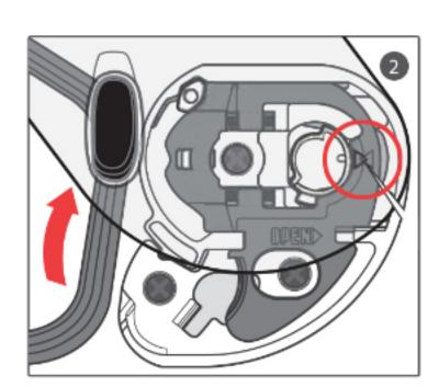
2. Open shield to the maximum open position.
