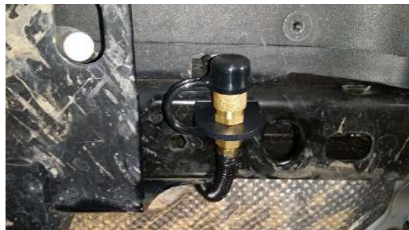
Figure 32 – Example of Air Coupler Mounted to Bumper
