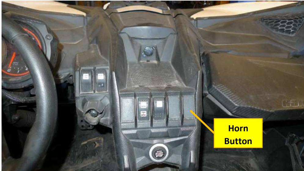
Figure 36 – Recommended install location for Air Horn Button
