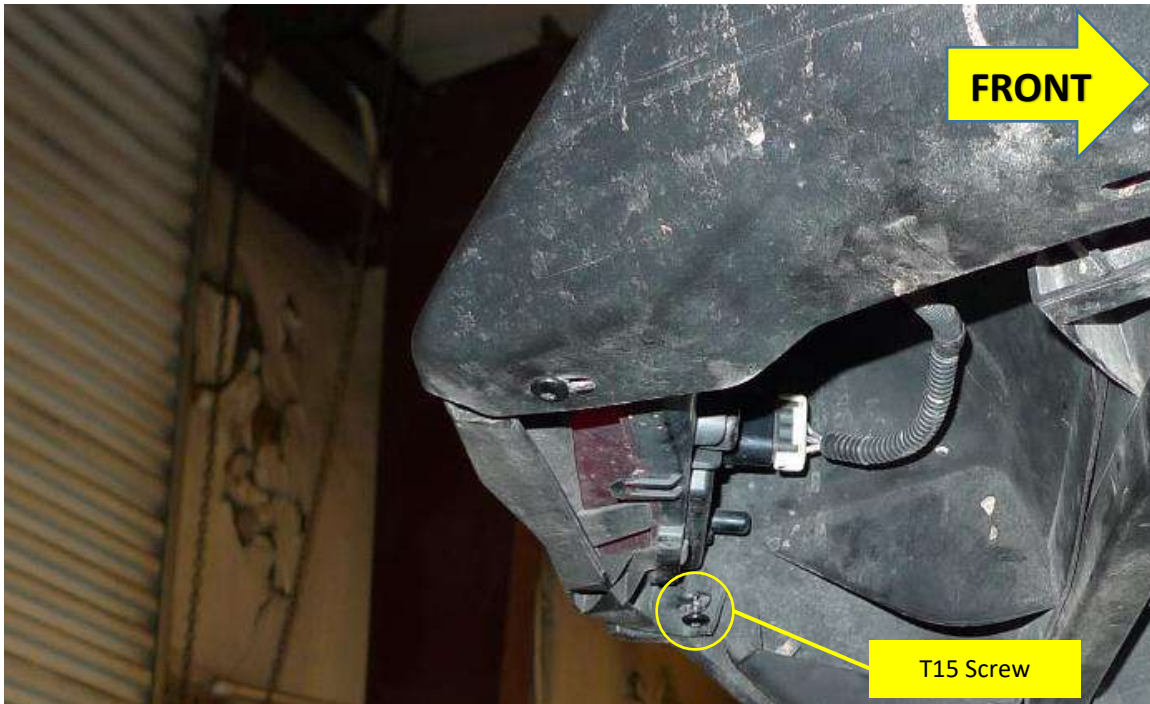
Figure 4 – Passenger Rear Fender Removal (below tail light)
