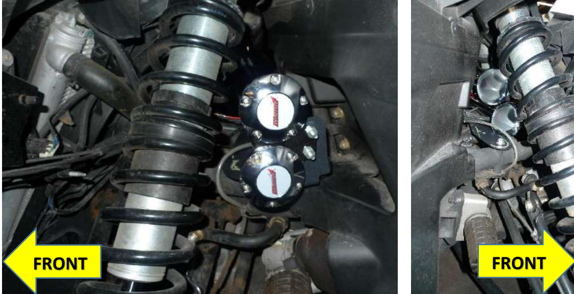
Figure 31 – Final installation of 102 Air Horn (X3 Turbo R shown)
