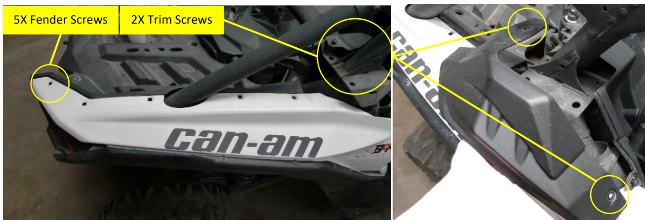
Figure 2 – Passenger Rear Fender Removal (fasteners on top of fender)
