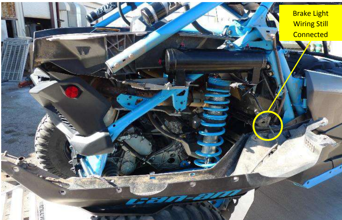
Figure 5 – Passenger Rear Fender Removal (fender resting on tire); Air Tank shown installed
