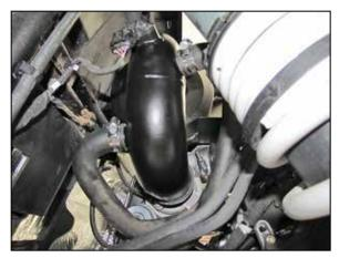
22. Install the K&N<sup>®</sup> intake tube into the coupling hoses, align for best fit and then secure with the provided hose clamps. Reconnect the inlet temperature sensor electrical connection and connect the BOV hose and crank case breather hoses. Secure the hoses with the provided hose clamps.
