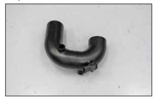
21. Install the inlet temperature sensor into the  $K\&N^{\odot}$  intake tube and secure with the provided hardware.
