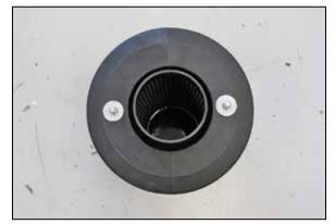
15. Install the filter assembly into the K&N<sup>®</sup> filter canister and secure with the provided hardware.
