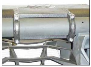
11. Secure the K&N<sup>®</sup> fresh air system to the chassis bar with the provided clamps and hardware.
