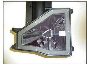
8. Install the provided gasket onto the lower portion of the factory fresh air housing and then install the K&N<sup>®</sup> fresh air system and secure with the hardware provided.
