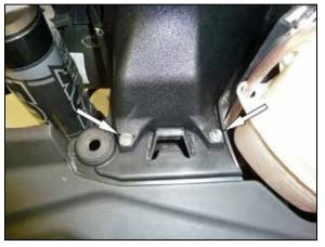
10. Install the K&N<sup>®</sup> fresh air system and secure with the provided hardware.
