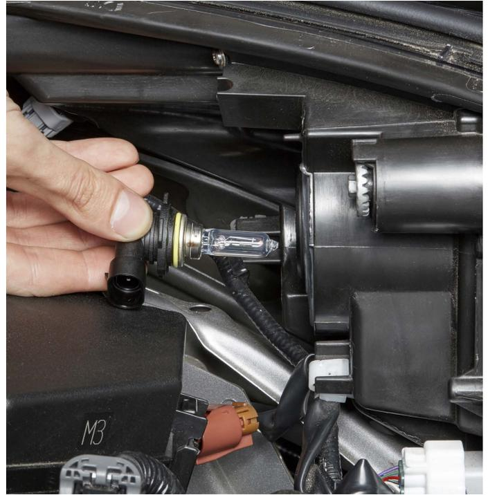
**STEP 4.** Place the new G10 LED conversion bulb in the socket and make sure it is secure.
