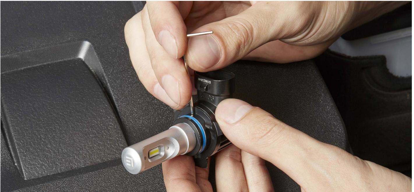
**STEP 7.** Once the bulb is properly situated, plug the bulb into the headlight harness. Do not re-install OEM dust covers, to allow for adequate cooling of conversion bulbs.
