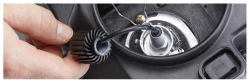
3 Secure the bulb in place using the clip on the headlamp assembly.
