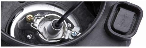
4 Screw the heat sink back onto the bulb
