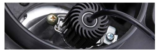
© Connect the red & black male connectors from the LED conversion bulb harness to the corresponding red and black female connectors from the headlight assembly (The wires from the headlight assembly may be connected inside the access hole – simply disconnect them and perform the step outlined above)
