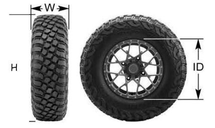
ATV tires are measured by Height (H) x Width (W) x Inner Wheel Diameter (ID), as shown in the above diagram.
