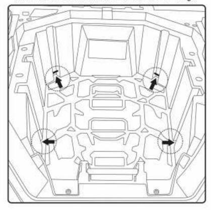
Using the supplied straps, pass around secure part of the vehicle, feed the strap through the loop end, and pull tight.
