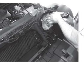
STEP 3: Remove the (4) T15 Torx Screws that hold the headlight trim ring bezel and lamp housing in place.
