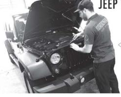
STEP 1: Open the hood and remove the (6) plastic rivets in the upper grill using a flathead screwdriver.
