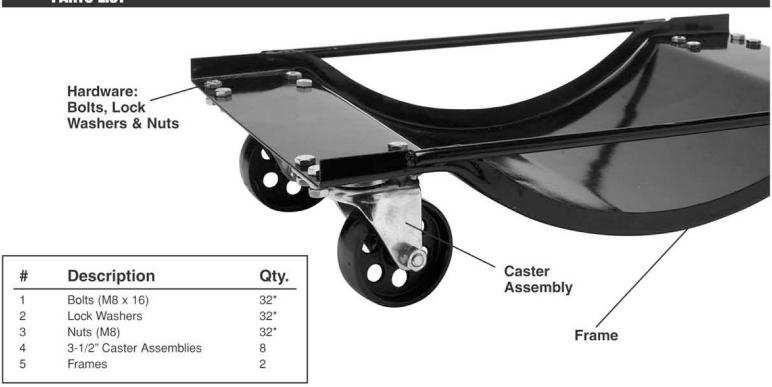
\* Replacements parts available in W54013HW Hardware Kit Replacement 3-1/2" Caster Assemblies available, part number W54013-1
