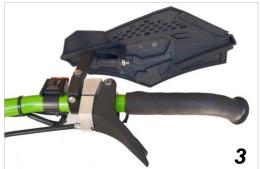
nut and tighten. This adjustment bolt is used to achieve the desired tightness of the mount. For now, leave the bracket loose so you can adjust the position up or down after attaching the handguard to the bracket.
