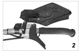
tightness of the mount. For now, leave the bracket loose so you can adjust the position up or down after attaching the handguard to the bracket.
