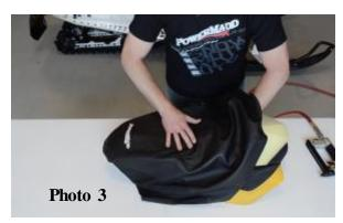
Step 7: Once you have placed 5-10 staples on the highest point, do the same on the opposite side and verify that the seat cover is still aligned correctly.
