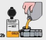
\*Check fluid level after 1-2 days. If consistency is low, have cooling system checked for leaks.
