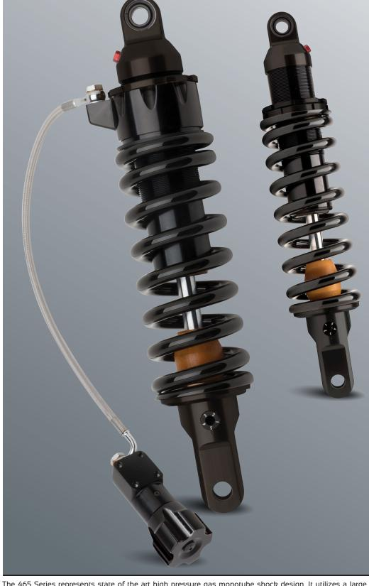
The 465 Series represents state of the art high pressure gas monotube shock design. It utilizes a large 46mm bore and deflective disc piston for precise damping. The beefy 16mm hard chrome shaft rides on custom viton seals for low friction and leak free life. Choose the R.A.P. (Remote Adjustable Preload) version that has a 5 position rebound adjuster that sets it up to perfectly match your bike, weight and riding style. Built in the USA.
