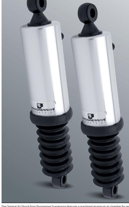
The Original Air Shock from Progressive Suspension features a machined aluminum air chamber for perfect sealing surfaces, heavy duty springs, air adjustability and velocity sensitive, multi-stage valving. The 416 Series is the perfect choice for the touring rider who carries a varied load. An optional adapter kit is available for most touring bikes to tap into the stock air fill system (fill valve or air compressor).
