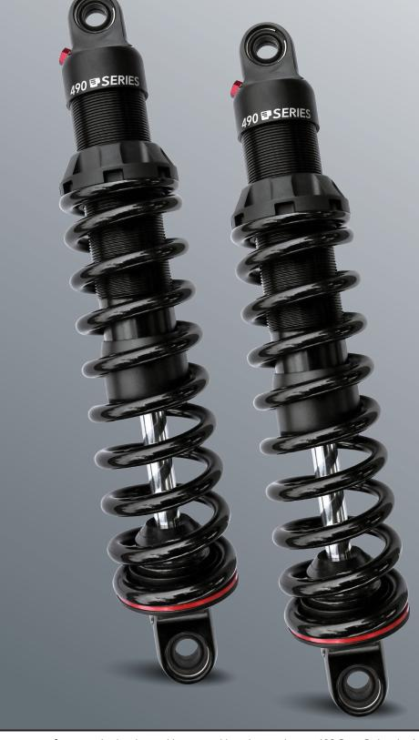
A true sport performance shock at heart with a competitive price tag, the new 490 Sport Series shocks feature a high-pressure monotube with deflective disc damping technology, hand threaded preload and a rebound adjustment to dial in the ride. An engineered jounce bumper with a built-in metal cup also help smooth out and control bottoming. From pounding the pavement around town to hammering around the tarmac on your next race day, the 490 is the perfect choice for your performance demand!
