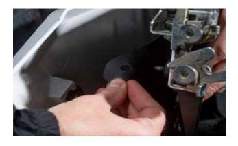
4. Line up the cut-holes on the bags liner, with the corresponding bolt holes on the frame and plastic panel. Re-install the bolts so that the bag is secured between the door's frame and plastic panel.
