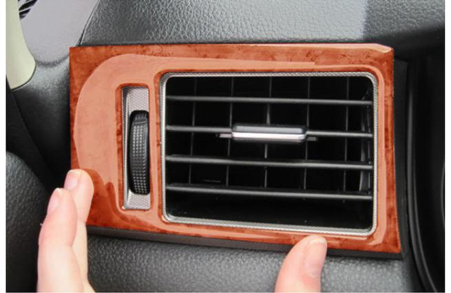
If any part looks damaged or doesn't fit properly, please contact CARiD right away. If you are installing a 2D kit, the test fitting process will also help you establish the areas where adhesive promoter must be used.
