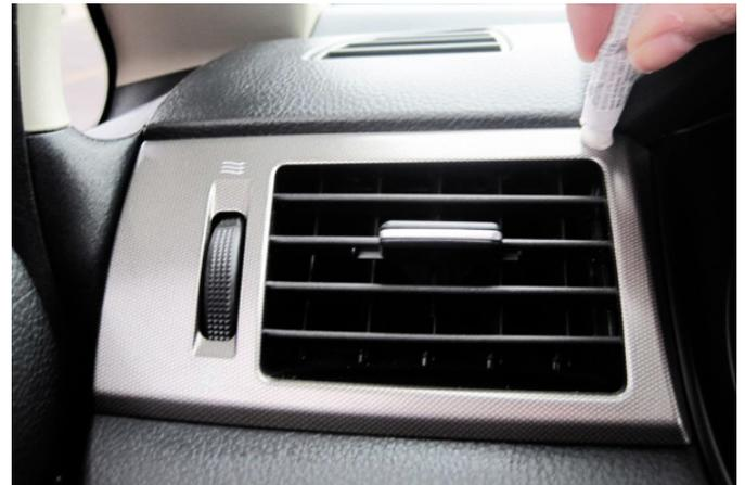
Thoroughly clean the dash surfaces where the dash trim pieces will be installed with isopropyl alcohol. These surfaces must be free of dirt and lint. Do not let the alcohol come in contact with any clear plastic surfaces covering gauges, clocks, radios or warning lights.
