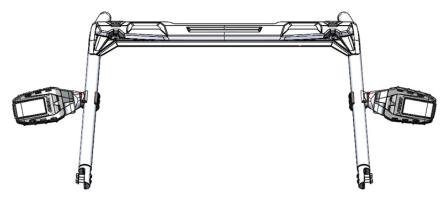
Reflect mounted on UTV cage with Wedge Washer in maximum downward tilt position.
