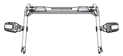
Reflect mounted on UTV cage with Wedge Washer in maximum upward tilt position.
