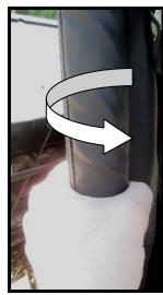
2. Locate the straps (wide and thin) running down the length of the rear vertical ROPS bar. Fasten around the bar. Repeat this step for the opposite side.
