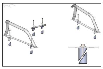
**3.** Attach the wedge nuts to the two basket side supports and center basket support using (6) M8x60mm bolts. Tighten just enough to hold the wedge nuts on.
