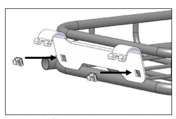
2. Insert the (4) Clip on nuts into the four holes on either side of the basket.
