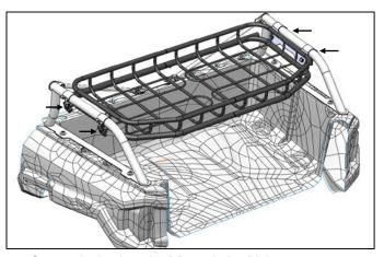
**8.** Secure the basket with (4) star bolts. Make sure to tighten all bolts before use. There are 6 securing the basket supports to the bed, and 4 securing the two support rods to the basket assembly.
