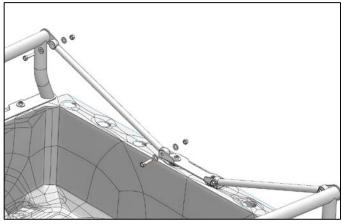
**5.** Attach the support rods with (4) M8 x 35mm Hex bolts (8) M8 washers, and (4) M8 Locknuts. Hand tighten bolts, but do not snug yet.
