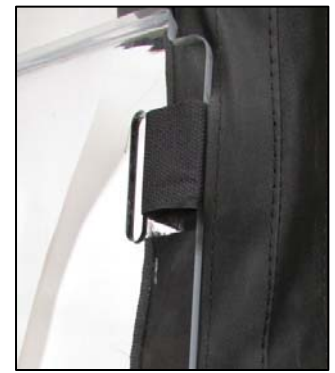
8. Install straps lacing through the flap opening to the inside of the cab & secure Velcro strap or P-Clamps. Reference Sezmik Versa-Shield Manual for Strap operation instructions..
