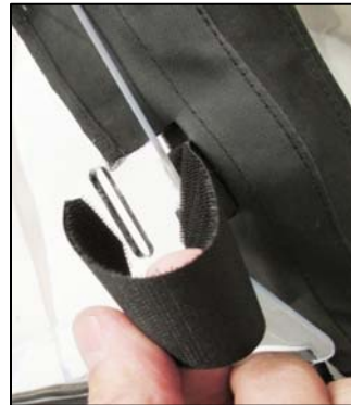
8. Install straps lacing through the flap opening to the inside of the cab & secure Velcro strap or P-Clamps. Reference Sezmik Versa-Shield Manual for Strap operation instructions..
