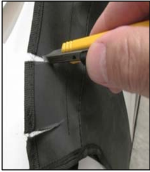
5. Cut 2 horizontal slits across the edge of the fabric to create tabs. Do not cut past the first vertical seam.
