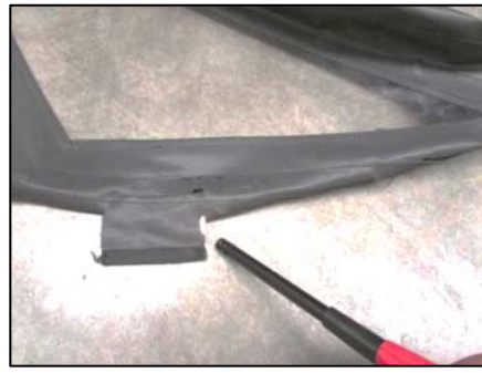
6. Mend the cuts with a lighter. Hold the flame on the material edge just long enough to melt the edge slightly. This will prevent the material fraying over time.
