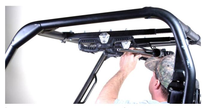
6. Open the jaws by releasing the rubber retention straps. Slide your gun into the jaws.
