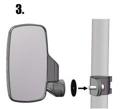
Screw the bolt into the mirror but do not tighten yet.
