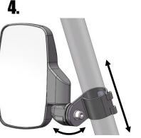
Slide mirror up or down Roll Cage tube to desired location. Rotate mirror on clamp to desired angle. When you are satisfied with the location and angle, tighten bolt.
