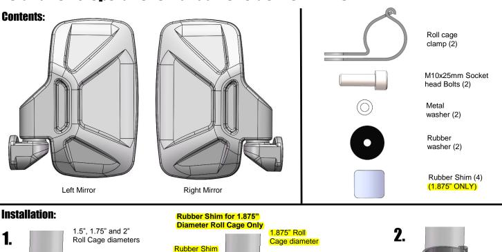
Open clamp and place around roll cage tube.
